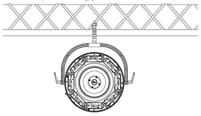
After fastening the product on a rigging structure, always secure the product with a secondary attachment in case of the rigging clamp fails.
